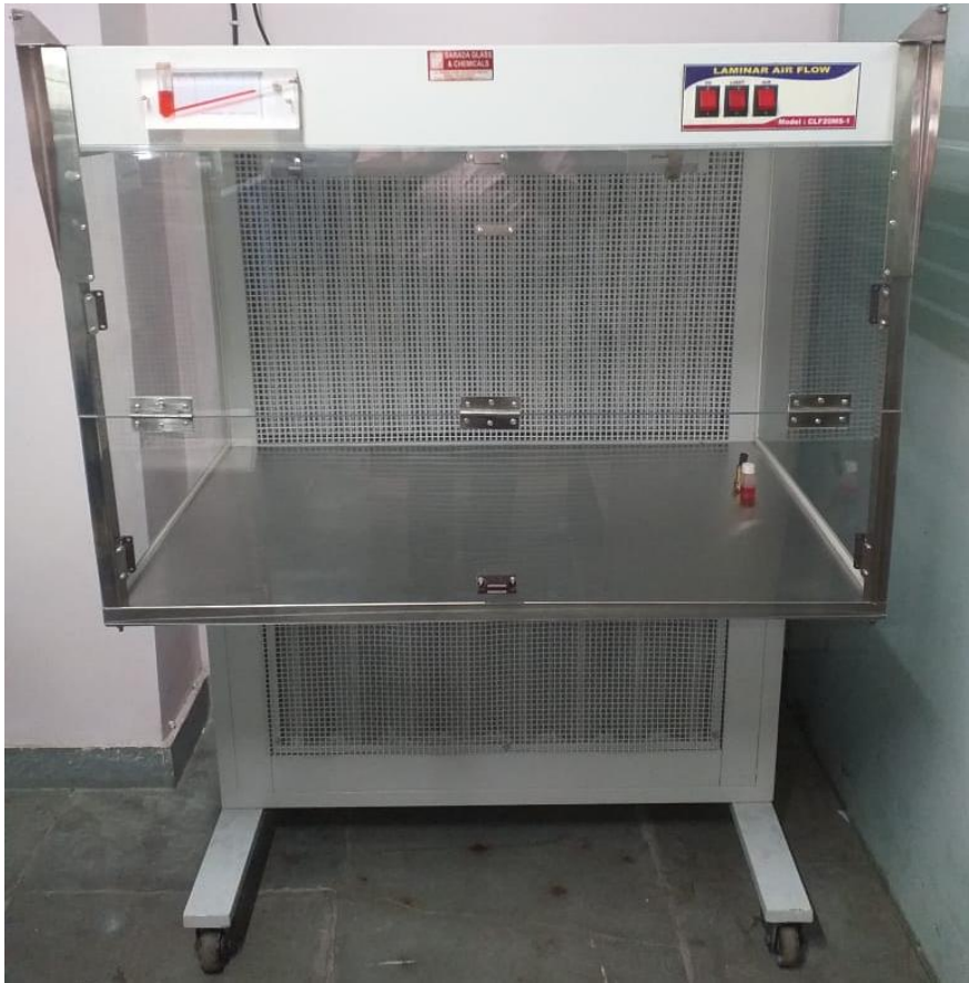
Name of the instrument: Laminar Air Flow Make: Sarda Glass and Chemicals
